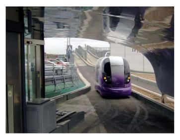
A Heathrow PRT 'pod' descending from the elevated guideway to a car park station.
