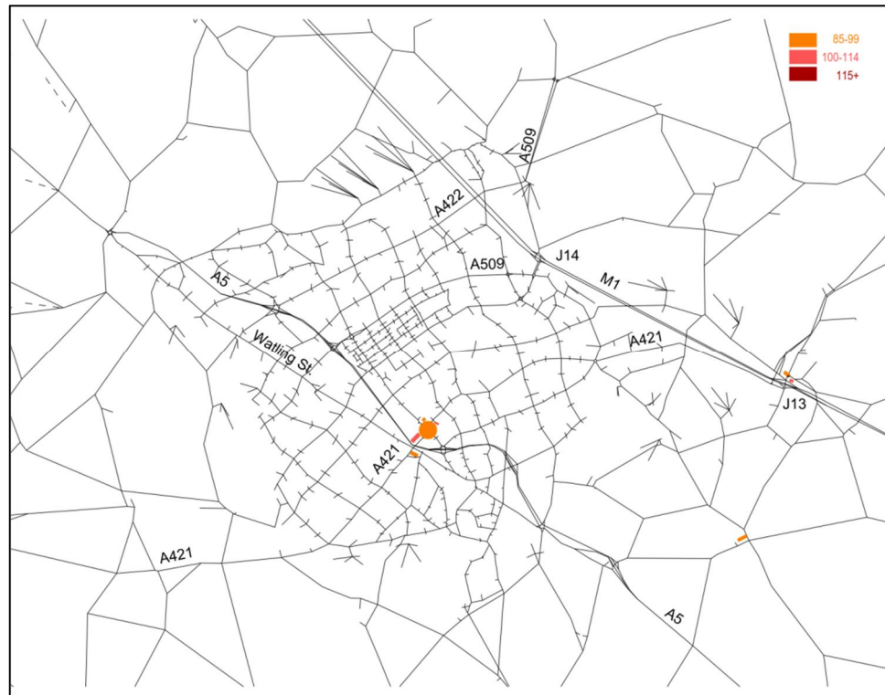
Figure 27. 2016 Base link and junction V/C over 85%, Inter-peak
