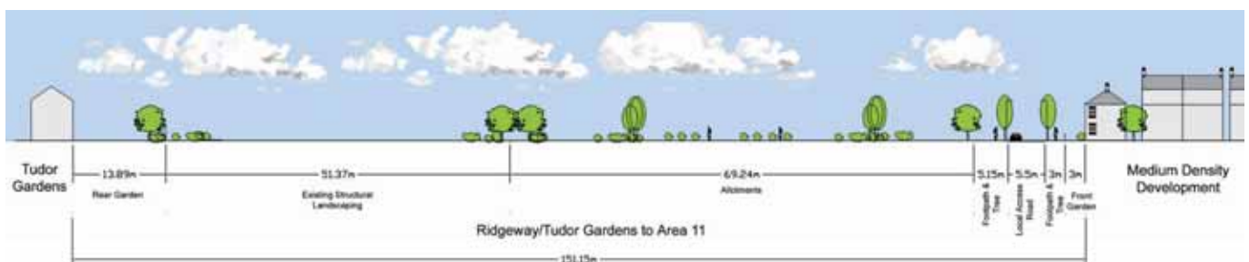
Figure 5.3 Section across open space and allotments from parcel M1 to properties on Tudor Gardens
