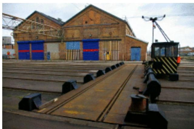
Picture 2.24 A works traverser
