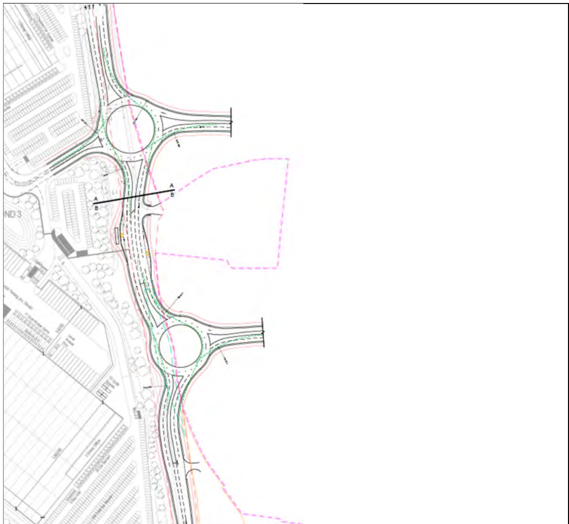
Figure 2: Preliminary Priority Roundabout Access Layout Northern and Southern Accesses
