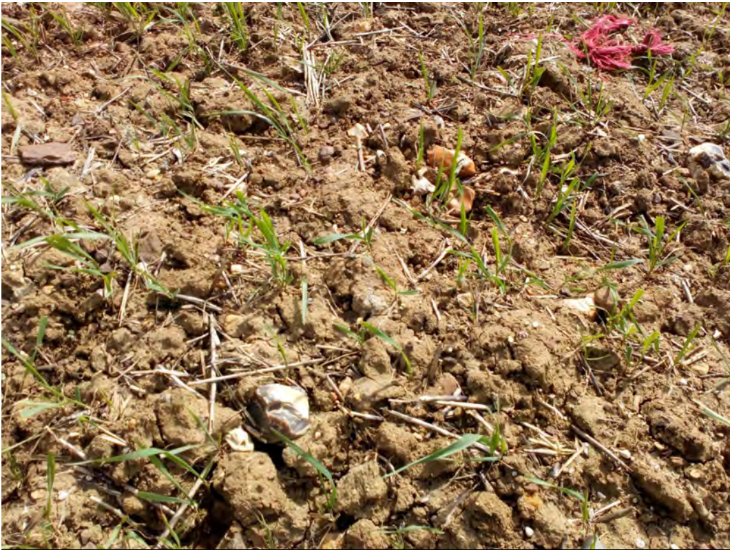
Photo 3 — Soils at the surface predominantly cohesive with angular to subrounded flint and chert gravel
