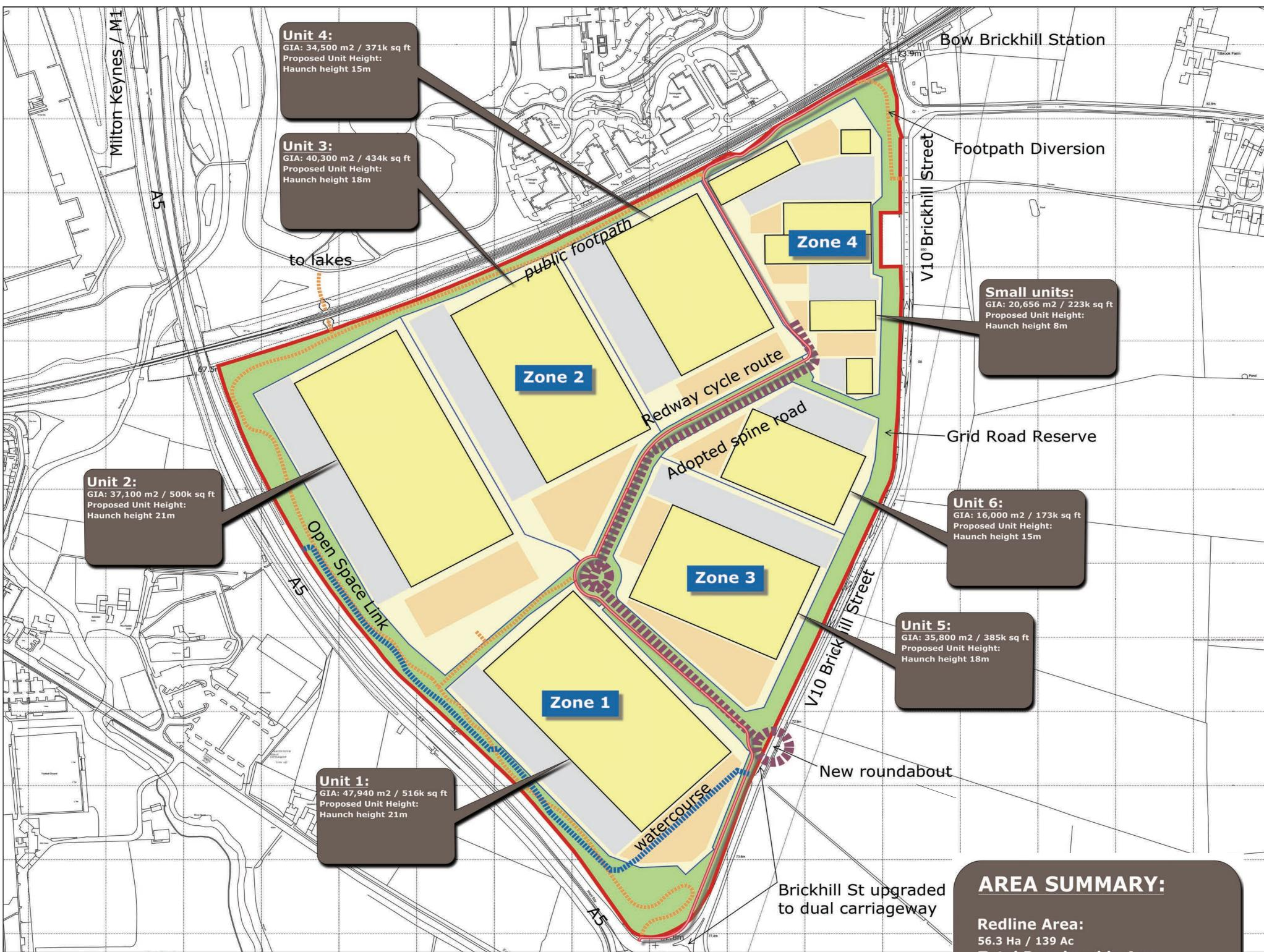
The above plan shows potential parameters for the development, including heights and floor areas. The proposals will compromise of 6-12 units with floorspace for flexible B2/B8 class use as well as ancillary B1(a) uses. Each unit will have its own surface water drainage strategy and the public realm will be attenuated. Landscaping will be included as part of the development proposals.
