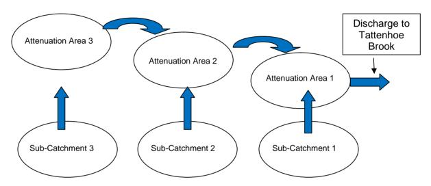
Figure 4 – Cascading Attenuation System Draining Sub-Catchments 1 – 3
