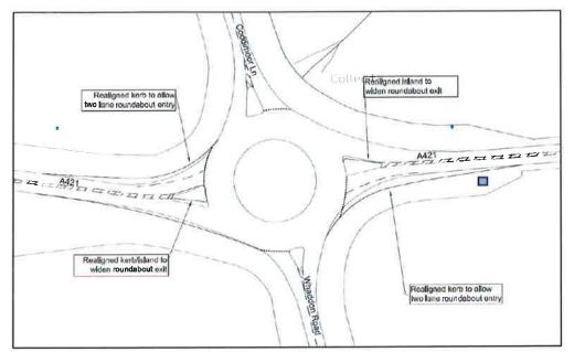
An independent Stage 1 Road Safety Audit has been carried out for the above scheme and the proposal was amended to ensure that the exit widths from the roundabout accord with standards set out in DMRB TD16/07.
