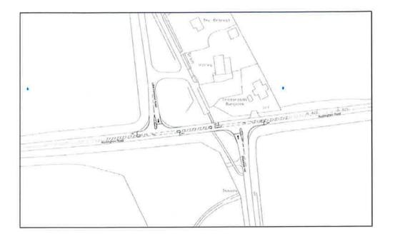
The proposed improvement to the A421/ Shucklow Hill/ Little Horwood Road junction has been modelled using LINSIG and the results indicate significant benefits in terms of queueing and delay on the minor road arms:
