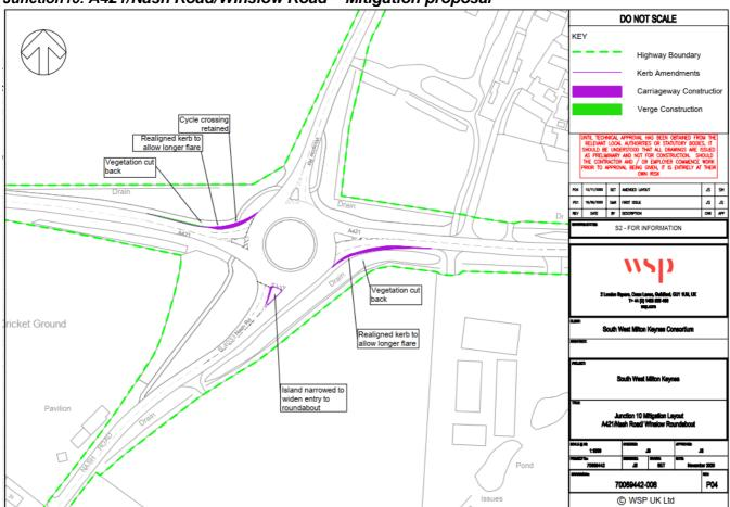
The proposed improvement to the A421/Nash Road/Winslow Road junction has been modelled using Junctions 9 (ARCADY) with the results detailed below.
