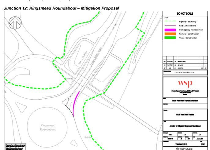
The proposed improvement to the Kingsmead roundabout has been modelled using Junctions 9 (ARCADY) with the previous capacity correction on Chaffron Way maintained as only kerb changes are proposed.
