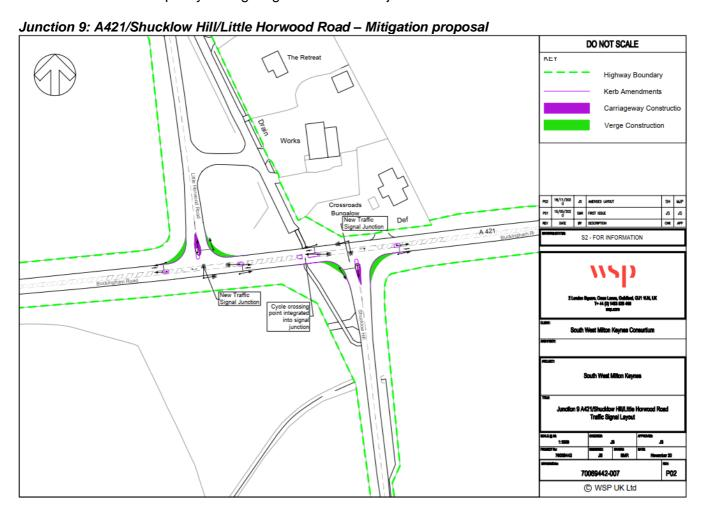
The proposed improvement to the A421/ Warren Road junction has been modelled using LinSig3 and the results indicate significant benefits in terms of queueing and delay on Shucklow Hill and Little Horwood Road in all the modelled scenarios. However, the signalisation of the junction would impose queues and delay on the A421 corridor with a queue of 24 predicted for the western arm of the Little Horwood side of the staggered crossroads.
