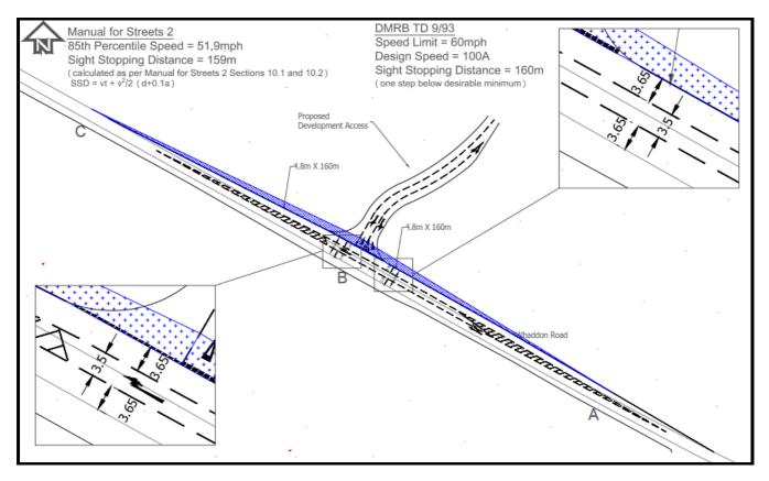
The Whaddon Road access junction has been modelled using industry standard software Junctions 9 (PICADY), as set out in TRN2. The results of the assessment show that the junction operates within capacity in both the AM and PM peaks for all the modelled scenarios with minimal queuing and delay expected, significant spare capacity is present to cater for possible increases in flow.
