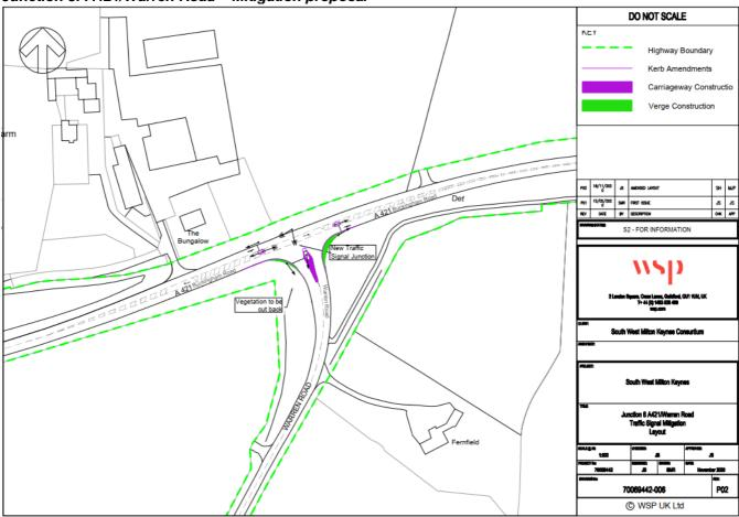
The proposed improvement to the A421/ Warren Road junction has been modelled using LinSig3 and the results indicate significant benefits in terms of queueing and delay on Warren Road in all the modelled scenarios, with the DS3 (including both SWMK and projected Shenley Park development traffic) have predicted queues and delay less than current 2020 results. However, the signalisation of the junction would impose queues and delay on the A421 corridor.
