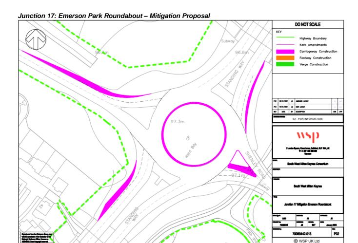
The proposed improvement to the Emerson Park roundabout has been modelled using Junctions 9 (ARCADY) with the previous capacity corrections were maintained as only kerb changes are proposed.
