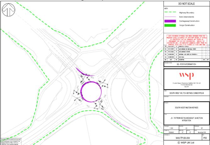
The proposed improvement to the Bottledump roundabout has been modelled using the industry standard LinSig software.
