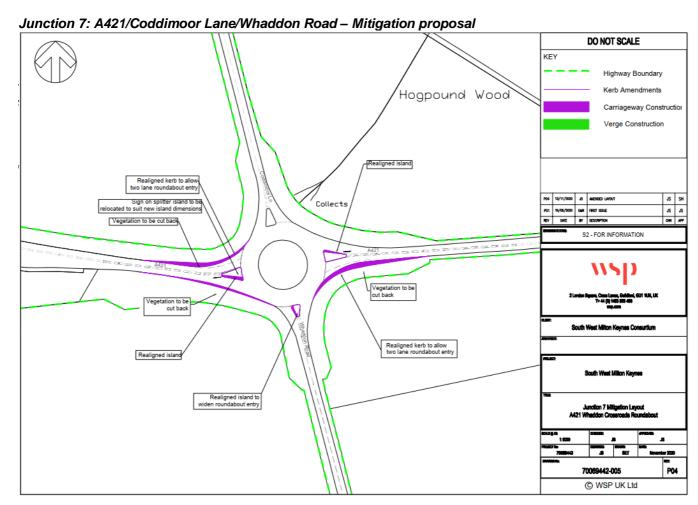
Junction 7: A421/Coddimoor Lane/Whaddon Road – Mitigation Capacity Results **Arm Description** ΑM PM Queue Queue **RFC** Delay (s) **RFC** Delay (s) (Veh) (Veh) 2033 Do Something 1 (Post-Mitigation) A - Coddimoor Ln 0.8 17.31 0.46 0.7 14.09 0.42 B - A421 (East) 3.7 8.91 0.79 4.2 9.39 0.81 C - Whaddon Rd 368.99 634.65 48.6 67.1 1.25 1.53
