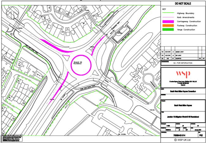
The proposed improvement to the Windmill roundabout has been modelled using Junctions 9 (ARCADY) with the previous capacity corrections were maintained as only kerb or road marking changes are proposed.
