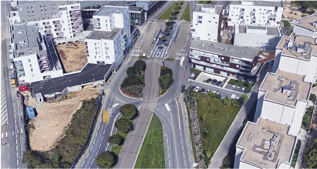
Figure 4-12: 'Hamburger' non-signalised roundabout junction in Nantes
