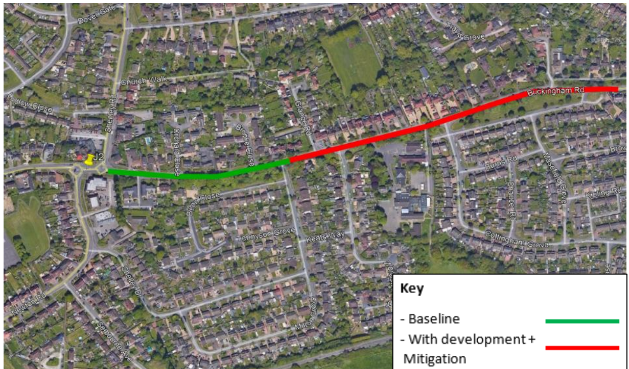
Figure 6.3: Junction 2 - Predicted extent of PM peak hour queuing
