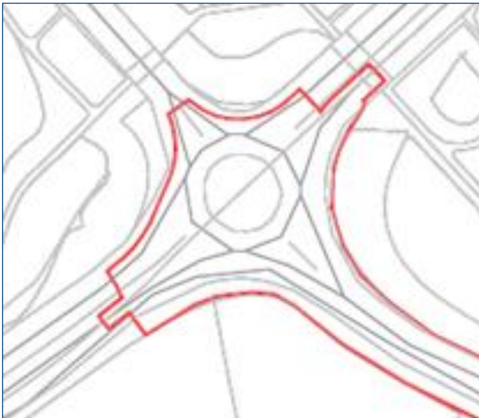
Figure 6.5: Planning red line boundary - NB that the proposed area of carriageway widening in the north of the junction lies beyond the red line
