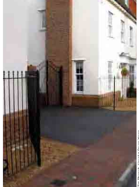
Figure 7.22 Beaulieu Park, Chelmsford: the visibility splays are provided by railings rather than boundary walls, although the railings could have followed the property boundary.
