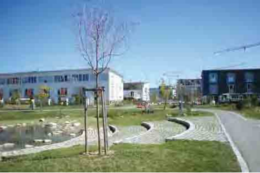
Figure 2.4 An example of a sustainable drainage system.
