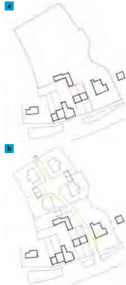
Figure 3.7 Small scheme design for an infill development (a) outlined in red. Location of new houses (b) shown in green together with new access street. Note that the new access street can be extended to allow for future growth at the top of the diagram.
