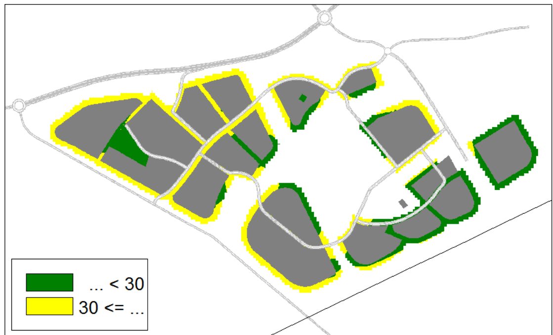
Figure 8.4 Night-time Internal Noise Level, dB L_{Aeq}
