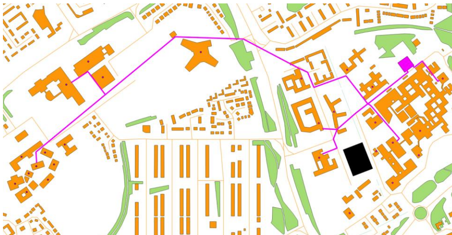
Cluster 4b (Hospital + Woughton) buildings and indicative pipework
