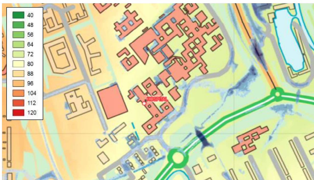
Figure 12 – Hospital flood flow route, flood map for surface water and LiDAR
