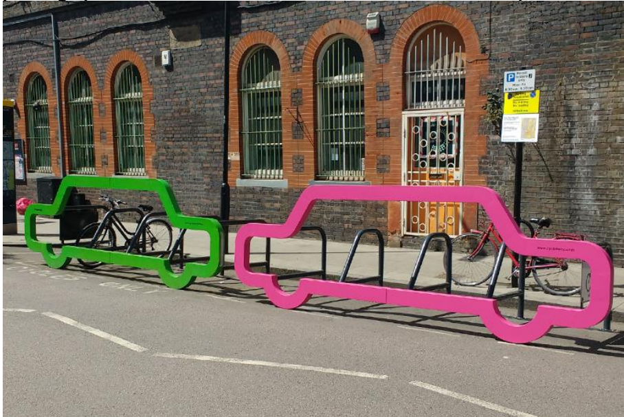
Figure 6: A bike port cycle parking solution that provides for 10 bicycles in a standard car parking space. The bold outline of a car demonstrates the space efficiency of bikes.
