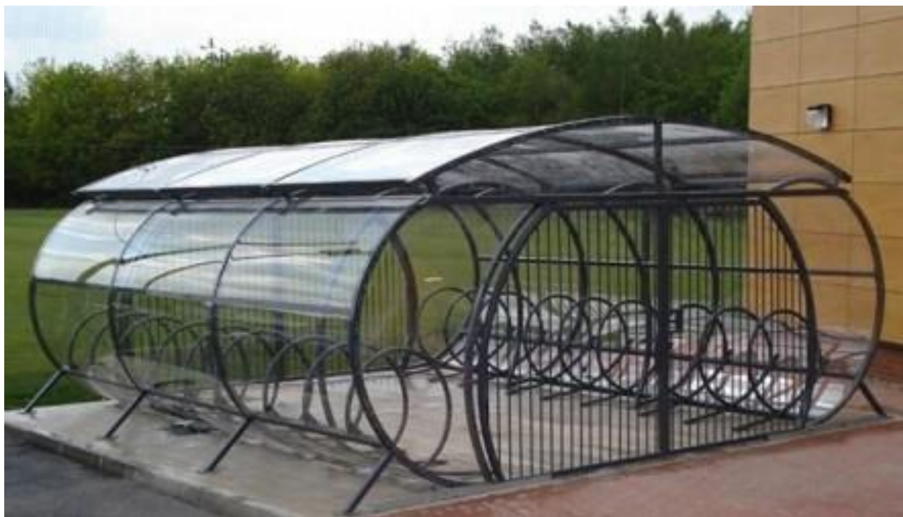
Figure 28 - Canopy style cycle parking (preferred option)
