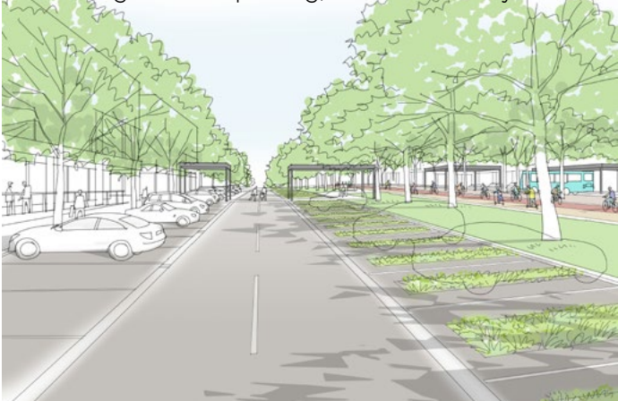
Step 1: Increase attenuation of surface water
