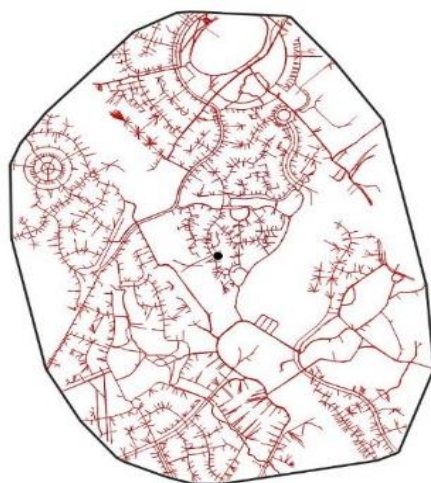
Figure 2: Example of route analysis conducted from an address point (black circle). The red routes extend 800m, and a polygon is drawn at their furthest point. This polygon is then checked if it contains each of the accessibility indicators listed in the table.
