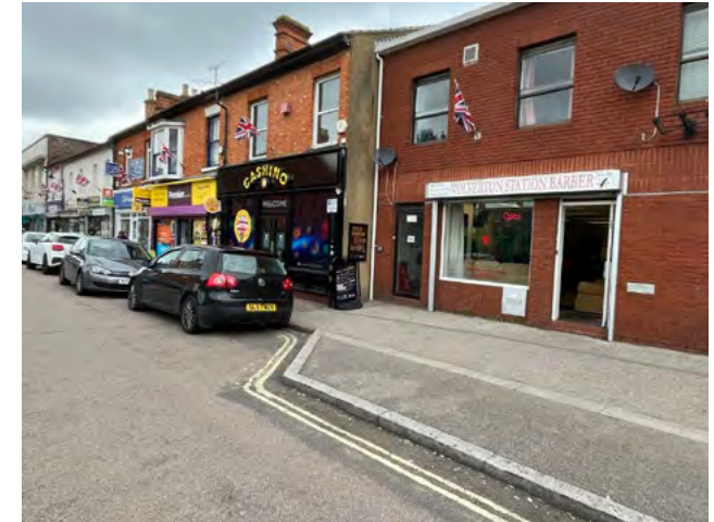
Figure 31: Build outs help to define parking bays.
