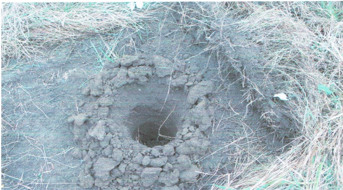
Photo No.5. One of the boreholes these were big enough for the strata to be identified and sampled directly.
