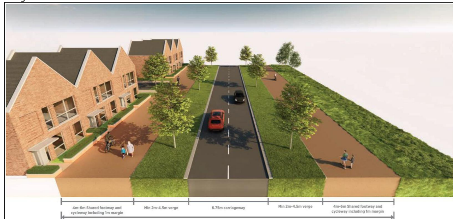
Image 15: Cross-Section of Local Roads
