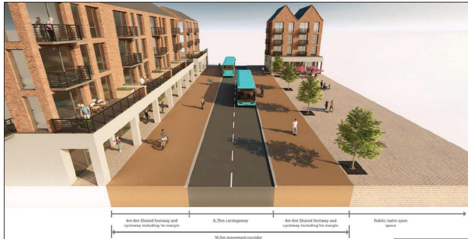
Image 14: Cross-Section of Primary Movement Corridor with Bus Lanes within Neighbourhood / Local Centres
